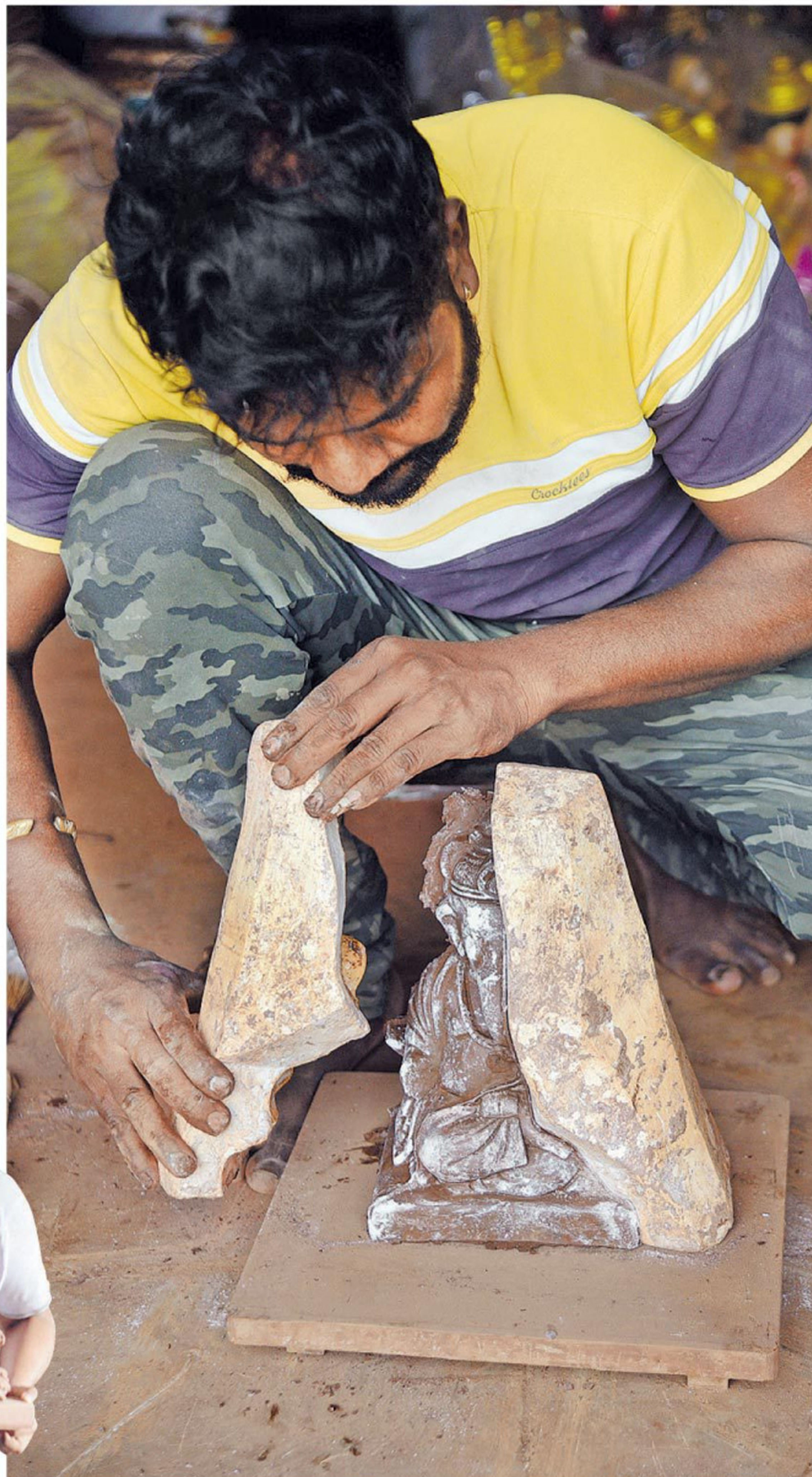
A karigar cracks open the mould to reveal a maati idol at a workshop in Uruli Kanchan, near Pune, run by Kedar Kumbhar and Dr Akshay Kauthale. The idols here are made from nothing else but farm soil and water. PIC/PRADEEP DHIVAR
